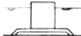
Caisson breakwater on rock foundation
