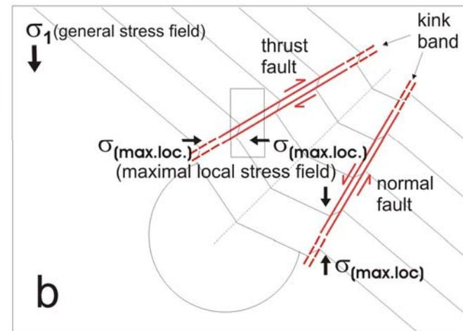
„Borehole closure“ due to bedding kinking combined with displacement along brittle fault zones.
