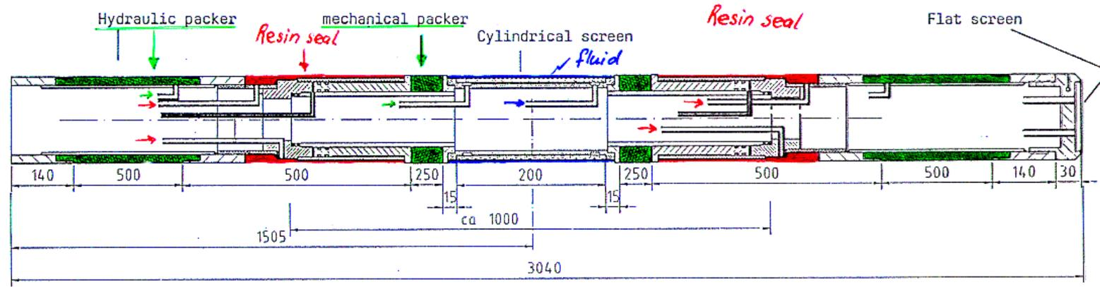
Principle of pore pressure measurements
