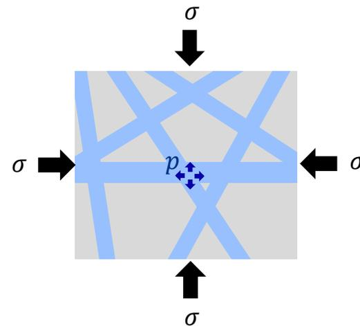
The effective stress  $\sigma^* = \sigma - \alpha p$  controls the opening of fractures
