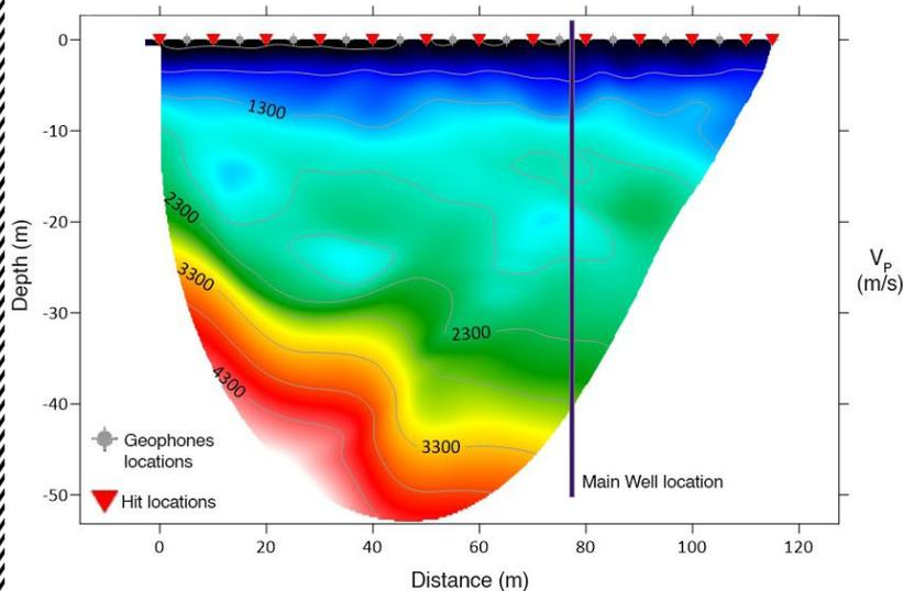
**B** - Refraction seismic profile - Grande Anse borehole
