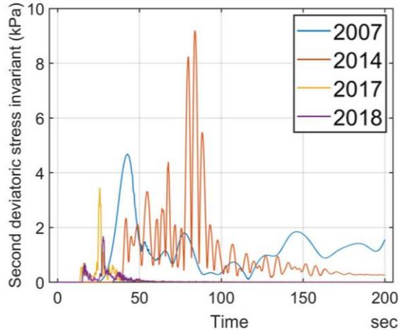
Numerical simulation of the seismic dynamic stresses at the borehole
