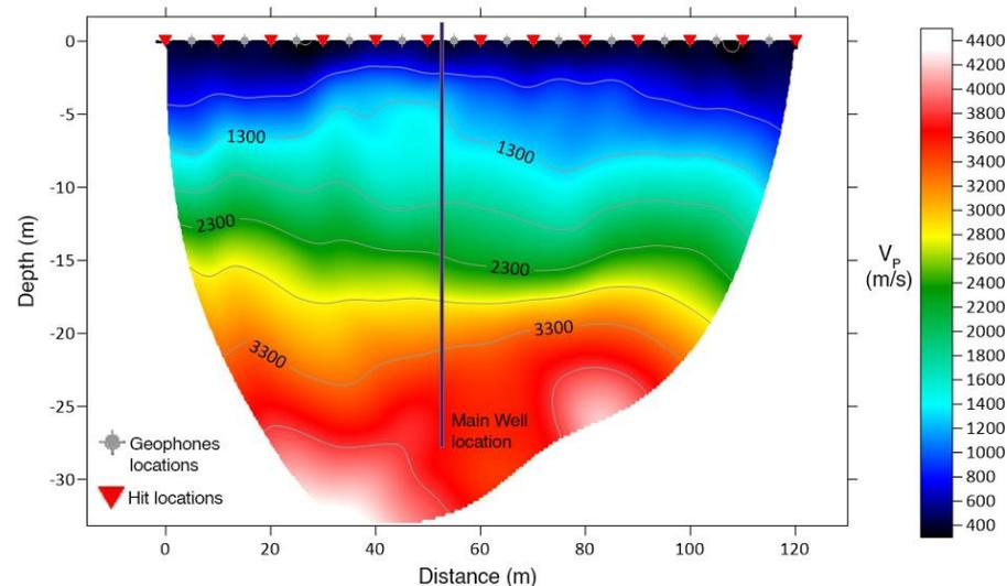
**Refraction seismic profiles ( $V_p$ ) around: A the Galion borehole, B the Grande Anse borehole. Well location and depth are represented by thin dark blue rectangles. The studied aquifers are located: between -20 and -50m at the Galion and -14 and -25.5m at Grande Anse.**
