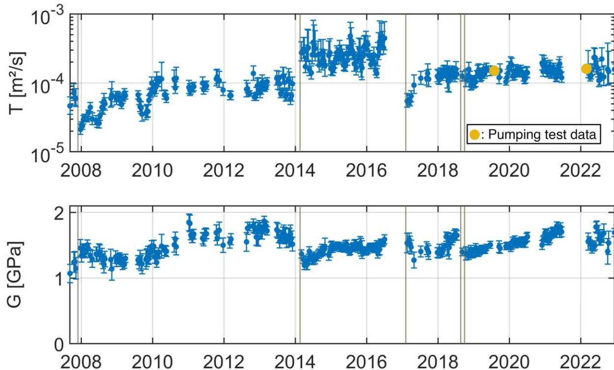
Shear modulus range validated with the seismic survey ( $G < 2\text{GPa}$ !)
