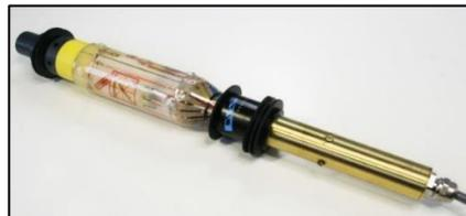
Csiro cells installed by Ineris
