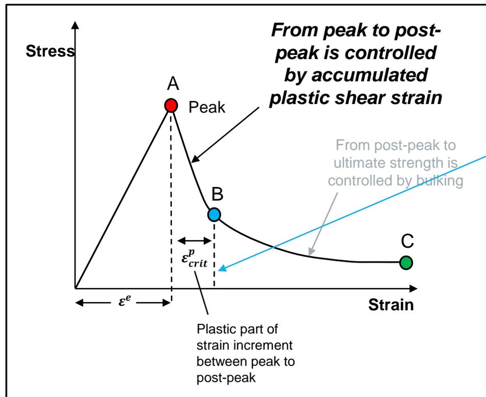
Critical Plastic Shear Strain:
