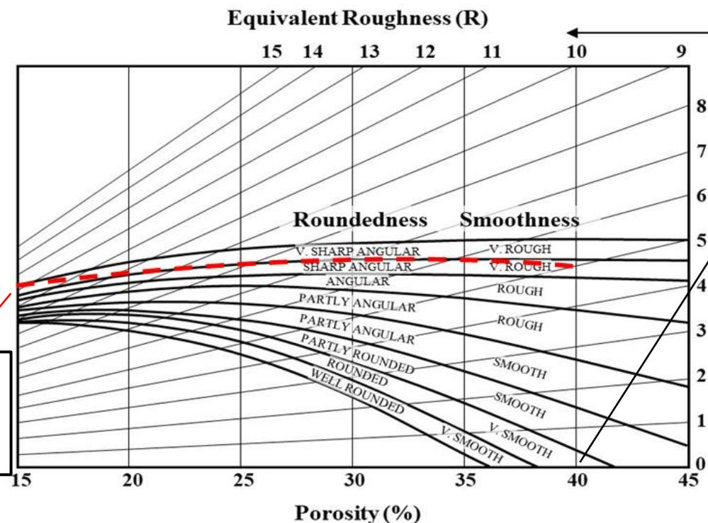
The **ultimate strength envelope** represents the true rock mass residual strength. At this point, the degree of rock fragments interlocking is at its minimum, and the **porosity is maximized** (maximum porosity of 40% is assumed).
