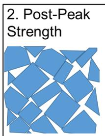
Ideally, the first and second residual envelopes describe the behavior of cohesionless perfectly frictional material with different degrees of interlocking.
