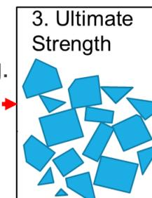
At **post-peak strength** the rock mass is assumed to have undergone fracturing, but the resulting **rock fragments are still fully interlocked** hence porosity is considered to be zero.
