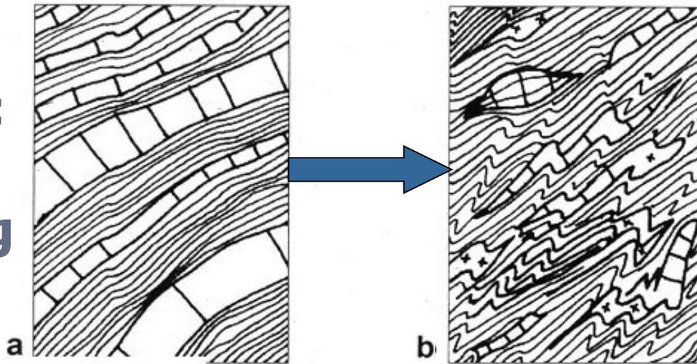
a. The seamy rock mass type consisting of intercalated rock members of strikingly different competence which are differentially deformed (sheared, folded and faulted)
