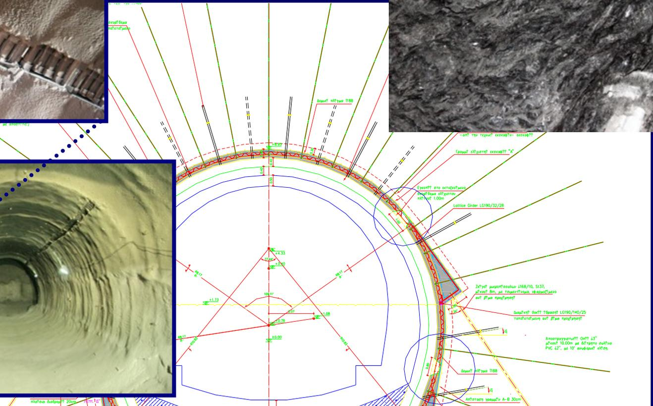
**Yielding primary support (sliding joints in steel sets and gaps in shotcrete) in very weak serpentinite (type IV) in areas of thick cover, 220m, GSI 15-20,  $\sigma_{ci}$  8MPa and  $m_i$  10**
