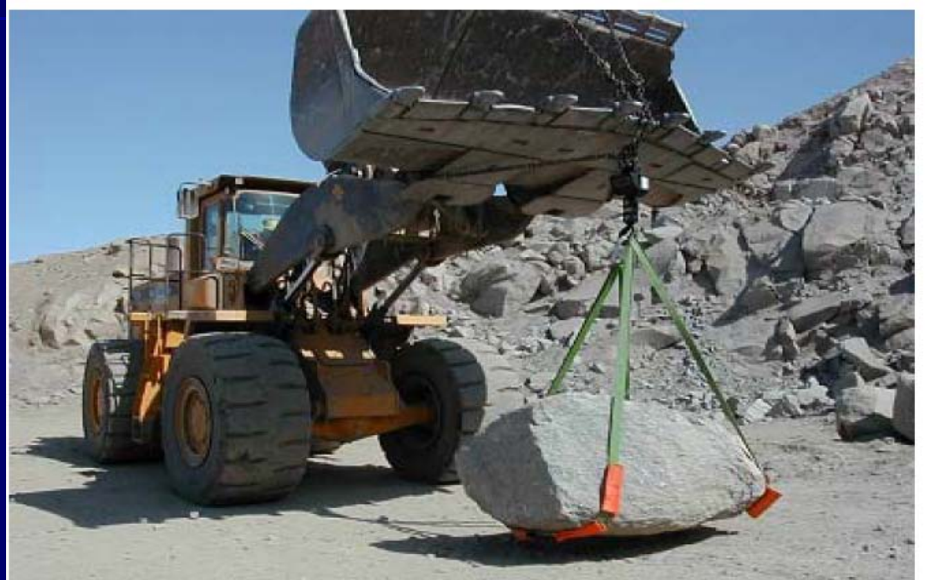
Figure 7: Wheel loader and 15 MT scale in weighing process.
