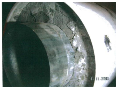
Fig 4.51: 4-1/2" ID Pipe with 16 lb/gal Slurry after De-bonding at 2,500 lb Force
